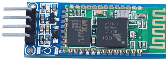
LED indicates Bluetooth connection status, flashing means there is no Bluetooth connection, constantly on means Bluetooth has been connected and the port has been opened.
